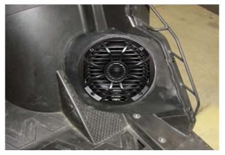
After attaching the speaker wires to the speaker install the speaker into the Wet Sounds kick panel.
