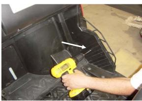
After marking the holes, drill them using a 1/4" drill bit
