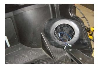
After securing all the allen bolts and the 7/16 nuts run your speaker wire into the speaker pod
